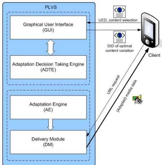
**Fig. 1.** System architecture of PLVS
